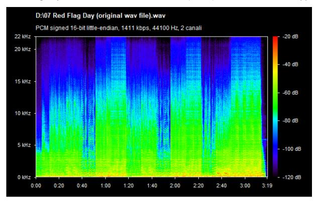
Converted file .WAV in MP3 320 Kbs quality (8MB), this is how the Spectrum Analysis appears
